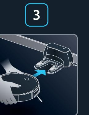
**EN** Position your robot on its docking station until the button is flashing red.
