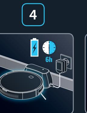
**EN** Wait 6 hours for the robot to be fully charged.
