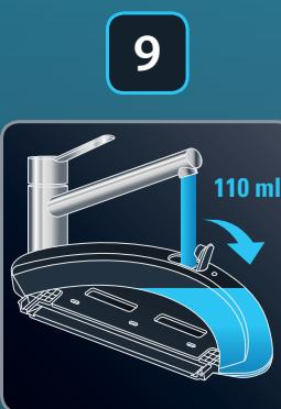
**EN** Open the water tank of the mop support and fill it with 110ml of water.
